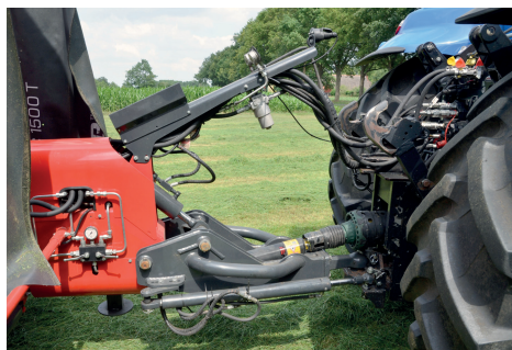
When the tractor turns, hydraulic oil from the cylinder on the drawbar is diverted to the cylinder on the 1500T's wheels.
