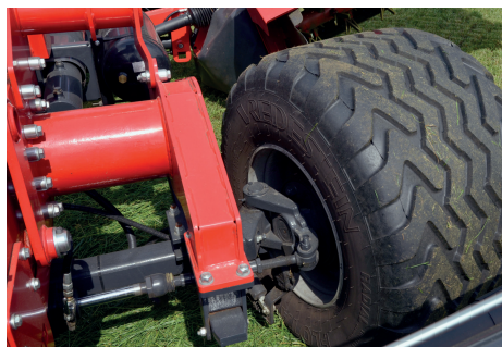
When the tractor turns, hydraulic oil from the cylinder on the drawbar is diverted to the cylinder on the 1500T's wheels.
