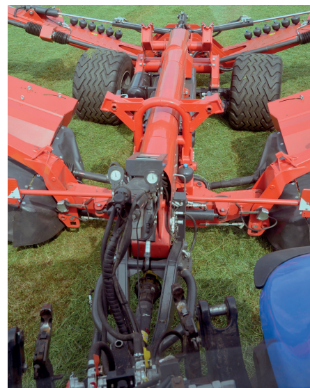
All hydraulic pipework and pto shafts are neatly concealed inside the main frame.
