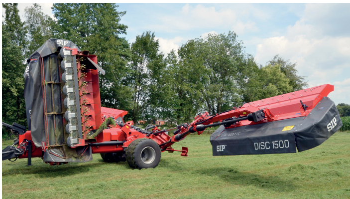
The two front mowers are raised vertically for transport, and secured in position by hydraulic locking pins. When folded, the two rear mowers rest on two V-blocks on the main frame. On-road dimensions are impressively compact, with a height of 3.99m and width of 2.99m.
