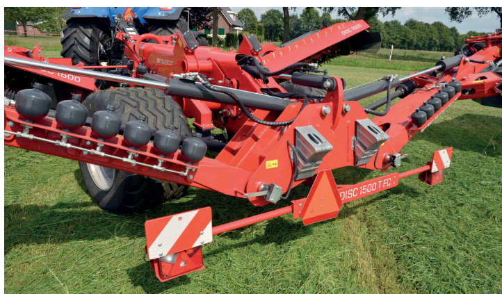
All five cutting units are equipped with hydro-pneumatic suspension to follow ground contours. Each rear cutterbar is relieved by six pressure accumulators and the front ones by two each side.
