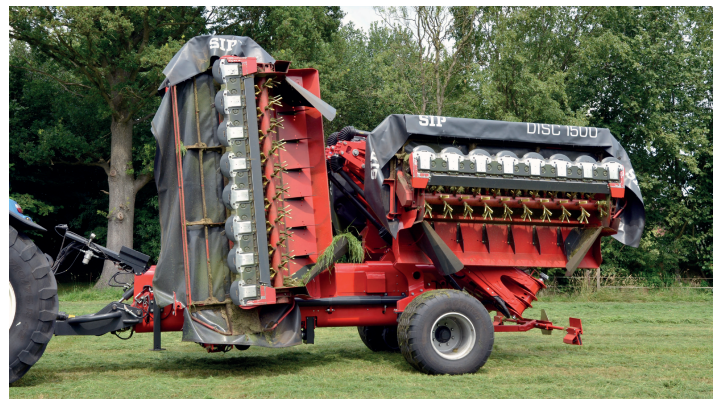
The two front mowers are raised vertically for transport, and secured in position by hydraulic locking pins. When folded, the two rear mowers rest on two V-blocks on the main frame. On-road dimensions are impressively compact, with a height of 3.99m and width of 2.99m.
